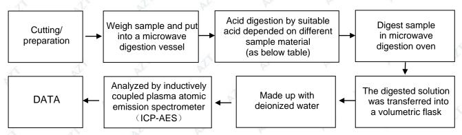
2. Test Flowchart for Cr6+ content (For non-metal material)
