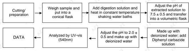
Test Flowchart for Cr<sup>6+</sup> content (For metal material)
